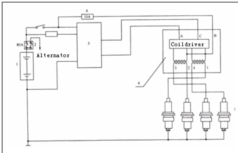
Fig. 9-2 Ignition system diagram (DELPHI)
