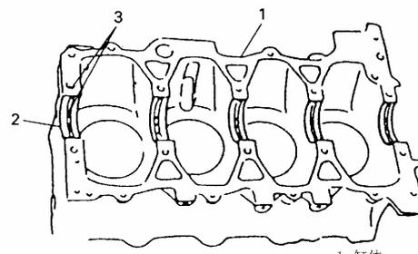
1. cylinder body 2. top main bearing brass 3. oil groove
