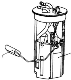
1. Fuel pump 2. Fuel level gauge float
