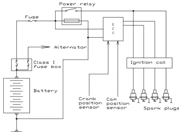
Fig. 9-1 Ignition system diagram (M 7 of UAES)
