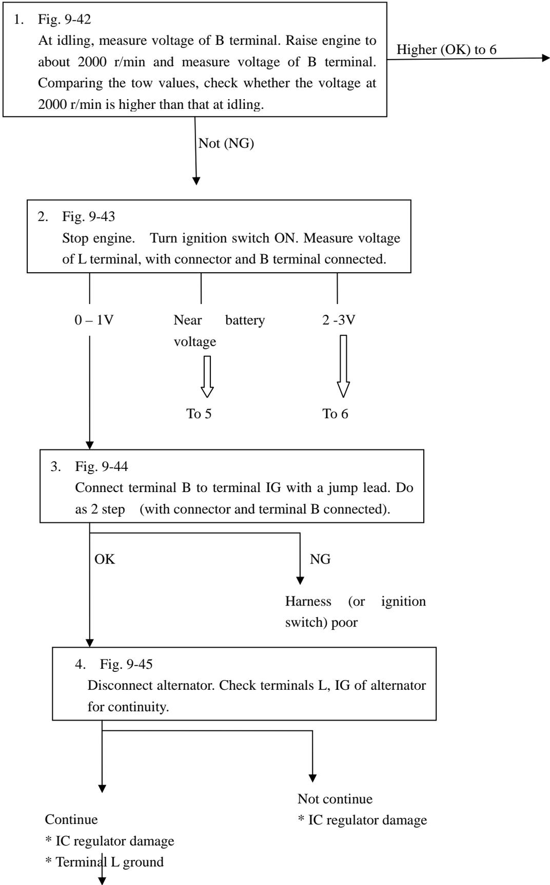
The Voltage is lower than the standard
