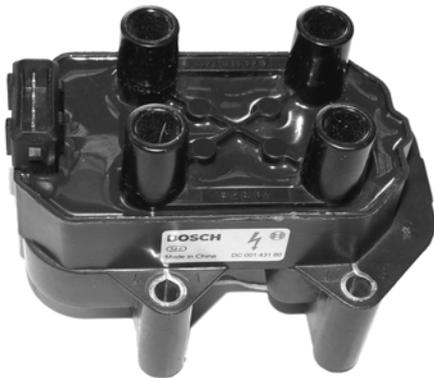
Fig.4-85 four post ignition coil
