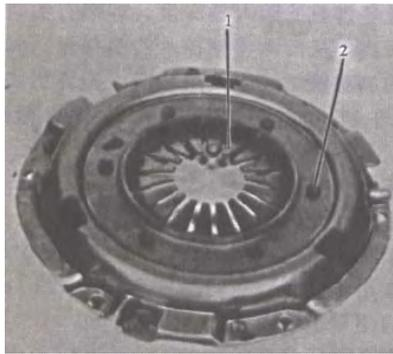
1- Wore diaphragm-spring tapering end 2-Rivet
