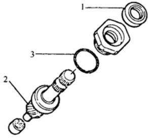
1- Seal; 2-Pinion; 3-Case seal ring
