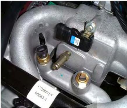
A device which is installed on the intake manifold stable pressure chamber to offer engine load.
