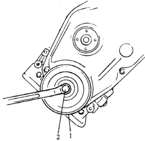
1 Crank shaft pulley 2 Crank shaft pulley bolt
