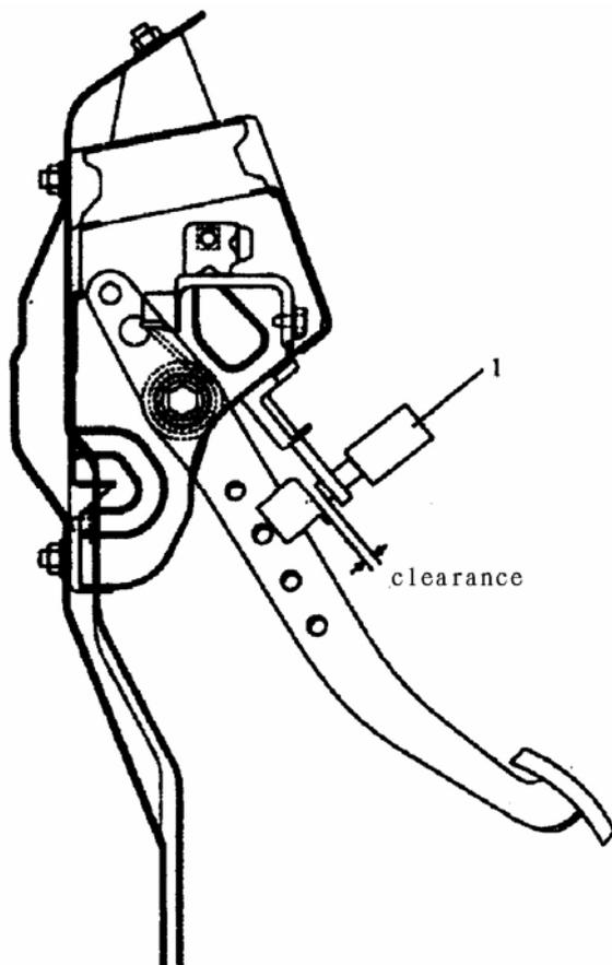
FIG.16-67 1.Brake Lamp switch
