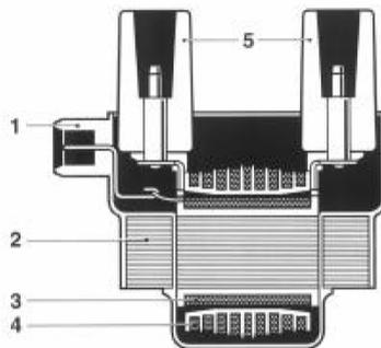
Figure 9-3 .Double ignition coil
