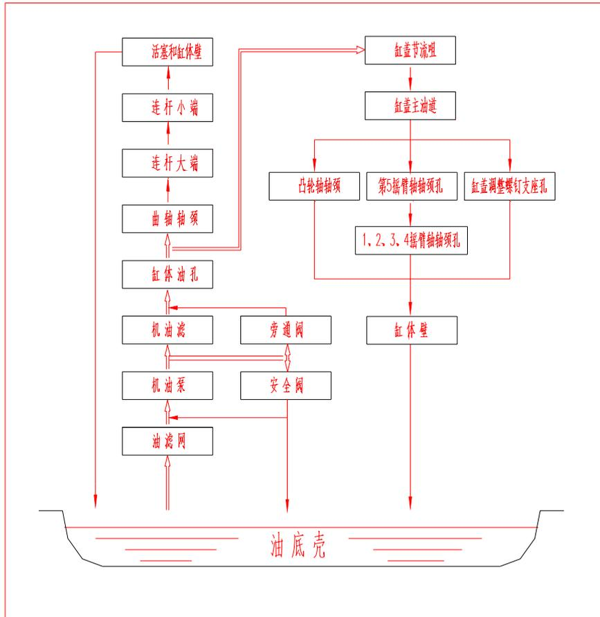
FIG.5-1 lubrication system main flow sketch map
