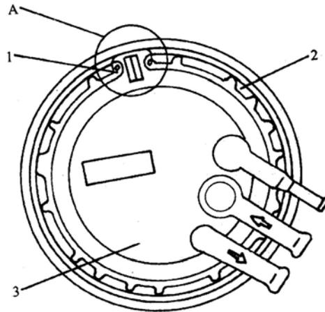
1. Clip 2. Fuel tank flange 3. Pump cap
