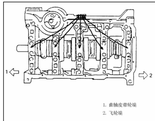
1. crankshaft pulley end
