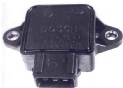
Fig. 4-77 throttle position sensor
