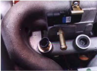
A device which is installed on cycling water route of inlet manifold, offers coolant temperature information to correct the amount of fuel injection and ignition timing.
