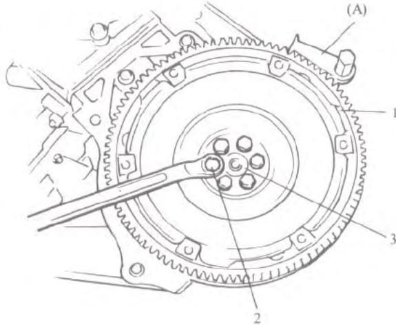
1-Flywheel; 2-Flywheel bolt; 3-Input shaft bearing; (a) Special tool (flywheel holder)
