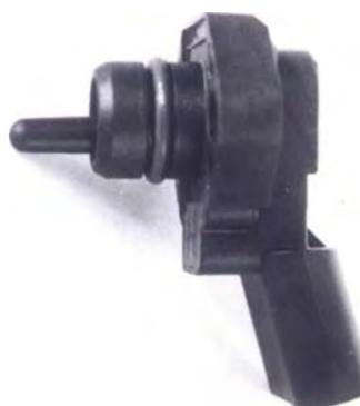
Fig. 4-78 intake pressure and Temperature sensor
