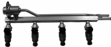
Fig. 4-84 fuel rail assembly
