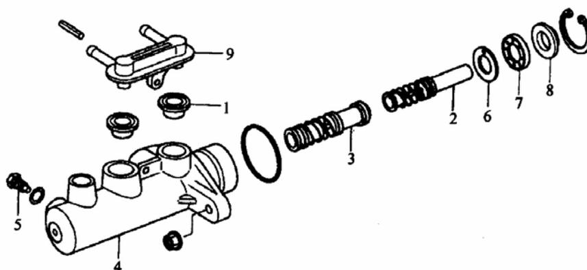
FIG.16-55 1.Seal bush 2. Primary piston assembly 3. Secondary piston assembly 4. Cylinder body 5.Stopper bolt 6.Washer 7.Cup 8.Stopper sealing 9.Pipe fitting
