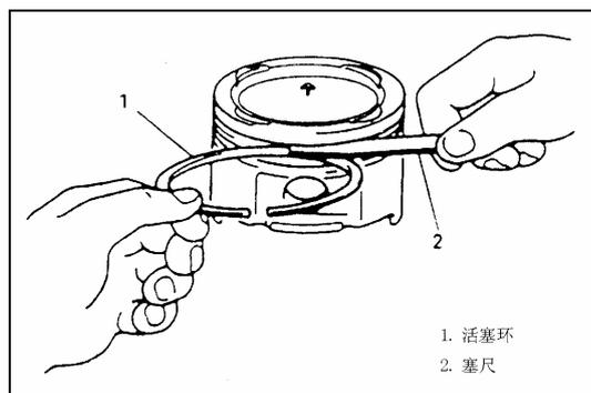
fig. 4-174 1. piston ring 2. Plug gauge
