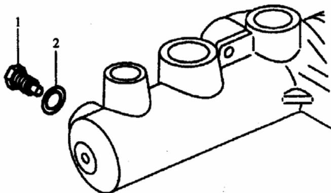
FIG.16-62 1. Stopper bolt screw hole 2. Secondary
